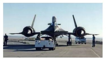
The nose attached just in front of the canopy. Due to a manufacturing defect, one of the noses fell off, and the crew had to eject. Another lost airplane was caused by a 2inch piece of duct tape which slowed down the instrument responses. The plane broke into pieces in midair.
