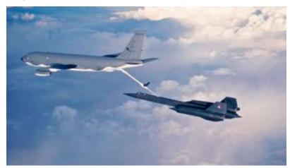
The plane used JP-7 which had such a high flash point that if you threw a lighted match on a puddle of fuel, the match would go out. On the ground, it leaked badly, and 55-gallon barrels were used to collect the drip. A little leaked during flight and collected in the body which expanded and sealed at cruising speed. The celestial viewing port was just in front of the fueling door, and a few had scratches.
